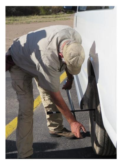
Keep tightening opposite lug nuts in a star pattern gradually in turn until each lug nut is as tight as it can be (the desired torque is 140 ft-lbs).
