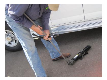
Consult the laminated instruction sheet that accompanies the jack for the best spot to put the jack. If the ground is muddy or very sandy, place the plywood square under the jack. Connect the ratchet wrench to the other end of the long tubes.
